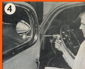
4 Press light through drilled hole, attach inside bracket, adjust frictions and the stop. Attach wire to ammeter. That's all there is to it!
