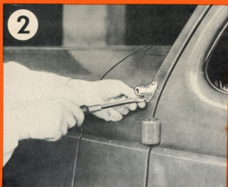
2 Position the bracket where you have marked location for the drill holes as indicated on the template.
