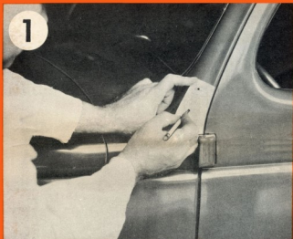
1 Position template enclosed with each FORD SPOTLIGHT in the manner shown above.
