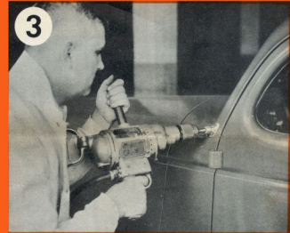
3 Put drill bushing in outside bracket and drill hole with 3/8-inch drill. The angle is pre-determined by bracket and drill bushing. Hold drill level.
